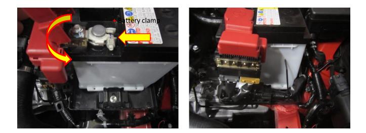
**9.** With the terminal tightened into its new position, you can now tidy the wiring loom, first tuck the excess loom around the back of the battery and cable tie it to the loom coming from the fuse box. Working backwards, cable tie the next part of the loom using the existing fastener hole.
