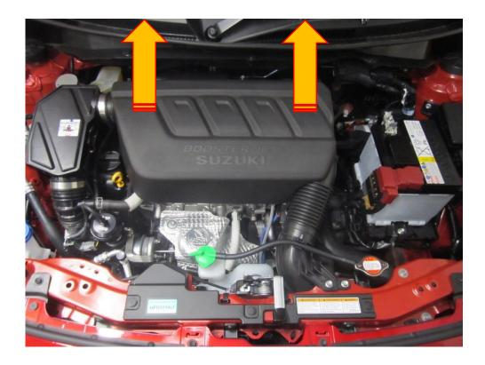
2. The air scoop/intake at the front of the engine bay is held down with four 10mm fasteners. These need to be removed with a 10mm socket and drive. You can remove the air scoop and hose (all three parts) from the engine bay.
