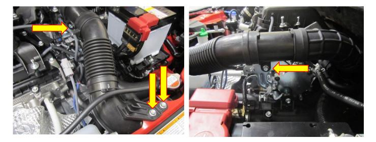
**3.** Locate the two 10mm fasteners attaching the air box to the engine, remove these with a 10mm spanner. Now remove the vacuum hose from the air box, this just pulls off.
